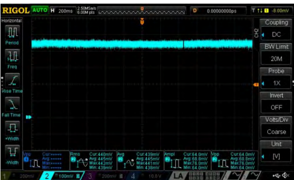
Figure 11: Roll-Ring Noise at 45RPM.
