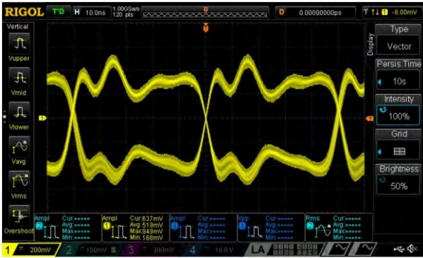
Figure 9: LVDS signal transferred through the Roll-Ring at 45RPM and 10 Mbit/s data rate.
