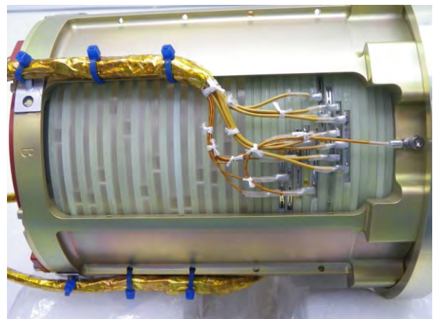
Figure 7: Routed Wire Harnesses on the 1075A Flight Model
